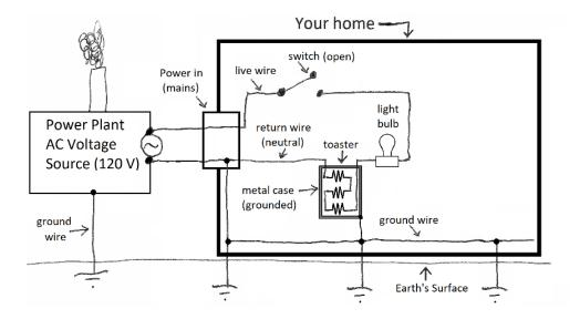
When the switch is closed (that is, the breakers are on), electric energy is provided to your appliances enabling them to function (the light bulb lights up and the toaster's internal wires heat up). Your home's wires now emit high levels of EMFs.
