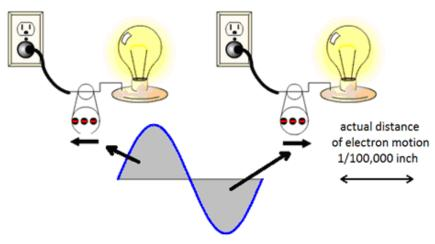
They wiggle back and forth, 50 or 60 times per second... that's a frequency of 50 or 60 Hertz...so fast that there is no real flow in one direction or another. Electrons move only about one hundred thousandth of an inch in each direction. It is this rapid back-and-forth movement of the electrons that keeps the lights on and makes toast out of bread. Keep this concept in mind as we now add you into the household picture.
